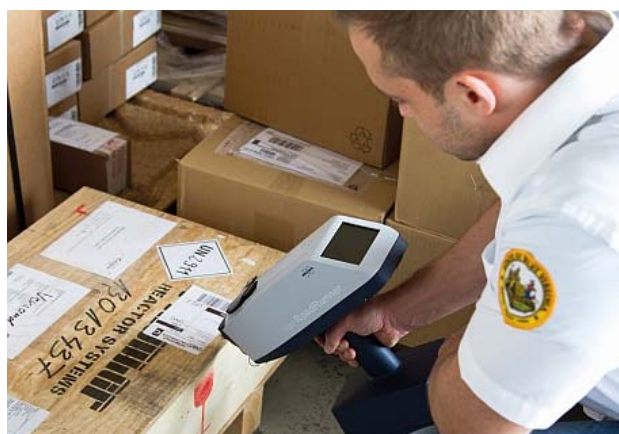
RoadRunner, a hand-held, battery-operated explosives and narcotics trace detector with outstanding performance.
