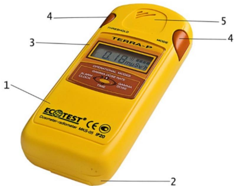
Figure A.1 – Main view of the dosimeter
